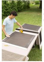
Cut an oversize piece of screening. Staple the screening to each of the six frames in this order, smoothing out any ripples before attaching: 12 to 6 o'clock, 3 to 9, 1 to 7, and so on, working around the frame. Cut any material that overhangs with a utility knife.
